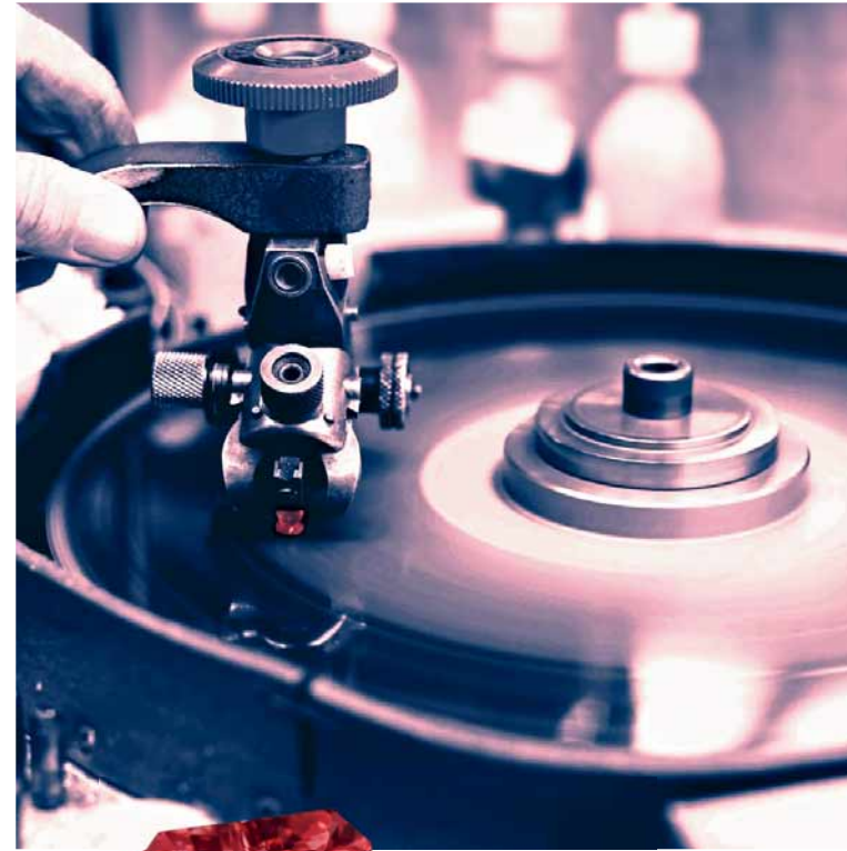
Clockwise from above: polishing wheel; rough pink diamond; pink diamond in a calliper during cutting and polishing; Argyle Cardinal; Linneys tiara (below)
